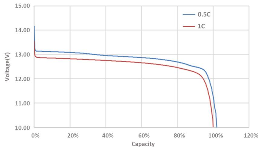
**80% DOD discharge curve after different cycles (0.5C standard charge)**
