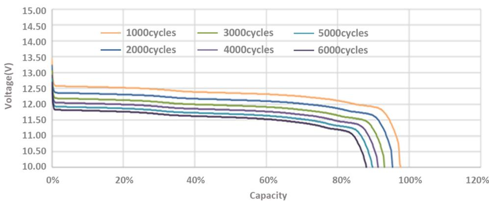
**0.5C charge and discharge cycle curve**
